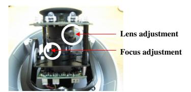
4. Lock the lens and tilt screws. Put the dome cover back and align the clear window in the dome cover with the lens. Attach the dome cover to dome base with the 4 mounting screws.
